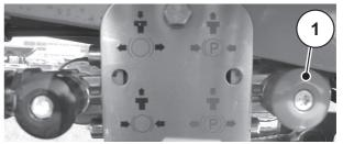
**1.** Push in valve [1] to release the parking brake.
