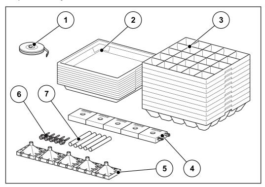
Figure 4.1: Scope of delivery of the field test set
