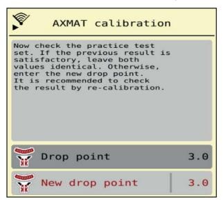
Figure 4.10: Performing AXMAT calibration
