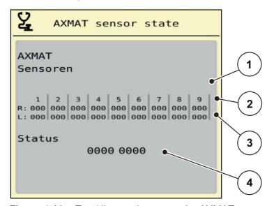
Figure 4.11: Test/diagnostics; example: AXMAT sensor status
