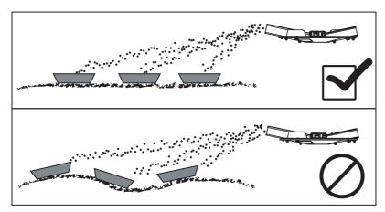
Figure 4.3: Layout of the collecting vessels
