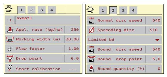
Figure 3.1: Fertiliser settings menu, tab 1 and 2
