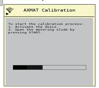
Figure 4.7: Performing AXMAT calibration
