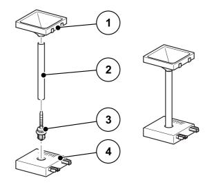
Figure 4.2: Assembling the measuring tubes
