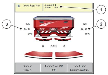
Figure 4.12: Regulating the drop point during spreading operation
