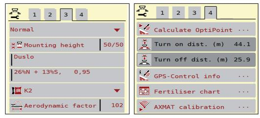
Figure 3.2: Fertiliser settings menu, tab 3 and 4
